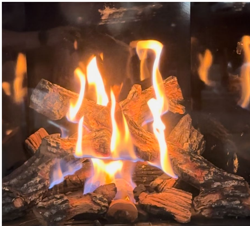
Figure 6-2 Burner Flame Heights: This image provides a visual reference for the burner flames burning at maximum height after the burners have been operating for 30 minutes or longer. A normal rear flame will be 1 to 2 inches above the rear log top edge. This, however, is dependent on the gas type, air shutter opening setting and vent system configuration. Actual flame heights can be slightly higher or lower when compared to this reference image.
